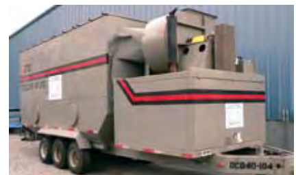
40,000-CFM mobile dust collector
