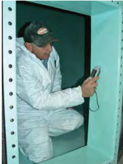
Checking mil thickness on internally lined vessel.
