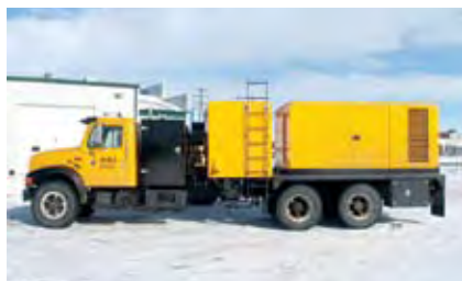
Blast unit cw 935 CFM compressor with Air Dryer and Air Purification System
