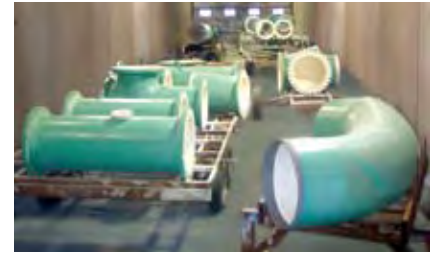
Pipe internals were coated with an NSF-approved potable water lining in our shop.
