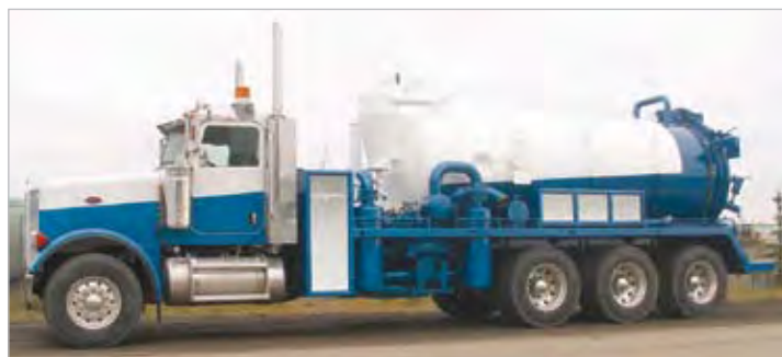
Vacuum truck - tank is internally lined with a protective coating. Exterior is painted with Endura®.
